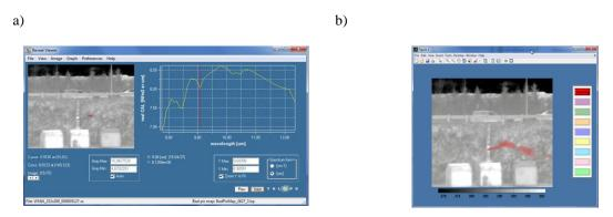
Fig. 12. The results of freon 134 measurements (concentration 3%, distance 60 m,  $T_{atm} = 18^{\circ}\text{C}$ ,  $v_{wind} = 8 \text{ m/s}$ ,  $p_{atm} = 992 \text{ hPa}$ ): (a) spectral characteristics, (b) results of analysis in Matlab.
