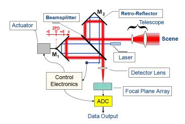
Fig. 4. Block diagram of imaging Fourier-transform spectroradiometer.
