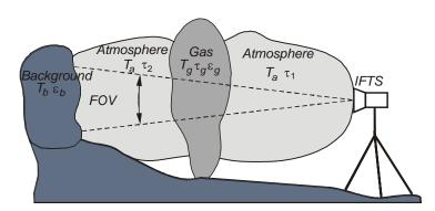
Fig. 5. Scheme of a measuring process and notations applied for the gas analysis in atmosphere.
