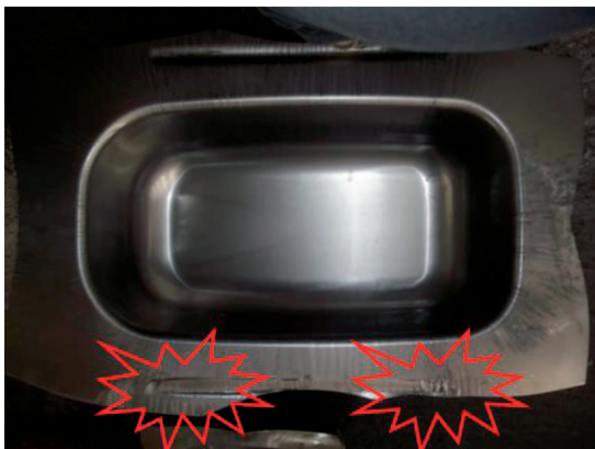
Fig. 15. Photo of final shape of a bathtub W1200 for the original die design with marked wrinkling area near geometrical drawbead
