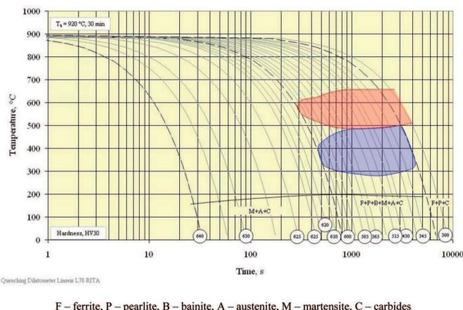
Fig. 12. CCT diagram of carbidic nodular cast iron with the composition: 3.72% C; 2.32% Si; 0.31% Mn; 0.50% Cr; 3.85% Ni; 1.03% Cu
