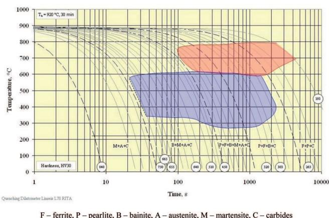
Fig. 6. CCT diagram of carbidic nodular cast iron with the chemical composition: 3.29% C; 2.35% Si; 0.07% Mn; 1.90% Mo; 0.94% Ni
