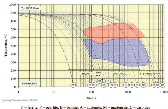
Fig. 10. CCT diagram of carbidic nodular cast iron with the chemical composition: 3.75% C; 2.40% Si; 0.33% Mn; 0.51% Cr; 1.41% Mo; 1.03% Cu
