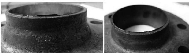
Fig. 13. Burr forming as result of bottom shearing
