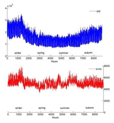
Fig. 1. Hourly values of active and reactive power consumption measured in TS 110/x kV/kV Sarajevo 5.
