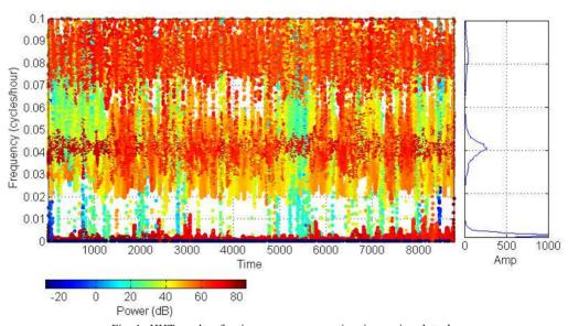
Fig. 4. HHT results of active power consumption time series plotted in time-frequency plane and Hilbert marginal spectrum.
