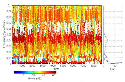
Fig. 6. HHT results of reactive power consumption time series plotted in time-frequency plane and Hilbert marginal spectrum.
