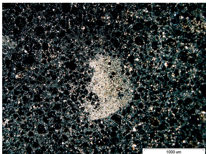
Fig.2. The micrograph of sample II, x nicol (grains of calcite, dark aggregates around calcite – brownmillerite)
