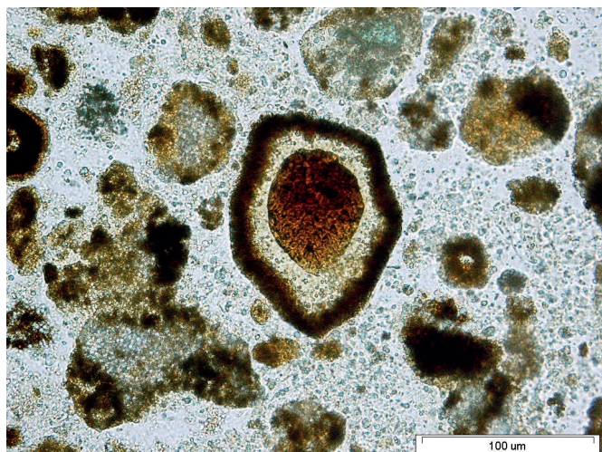
Fig.1. The micrograph of sample I, 1 nicol (grains of brownmillerite, outer built from brownmillerite and zone between them – periclasite)
