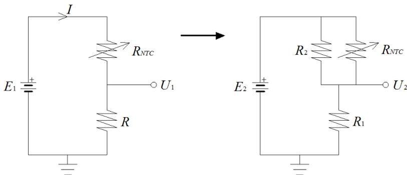
Fig. 2. Conversion from the serial voltage divider circuit (left) with a non-standard voltage source  $E_1$  to the serial-parallel voltage divider circuit (right) using a standard voltage source  $E_2 = 5V$ .
