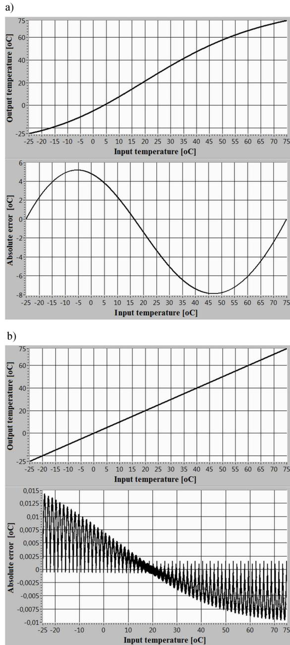
Fig. 6. The transfer function of the whole system and the absolute error [°C] for the temperature range from -25 to 75°C: a) before the linearization is performed by the two-stage PWL ADC ( $N_1 = 0$  bit,  $N_2 = 16$  bit); b) after the linearization is performed by the two-stage PWL ADC ( $N_1 = 6$  bit,  $N_2 = 10$  bit).
