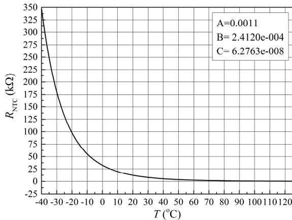
Fig. 1. The resistance-temperature relation of a NTSD0XV103FE1B0 thermistor.
