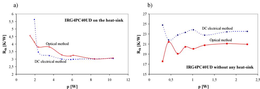
Fig. 3. The measured dependences of the thermal resistance of the investigated transistor on the dissipated power for the transistor a) placed on a heat-sink; b) operating without any heat-sink.
