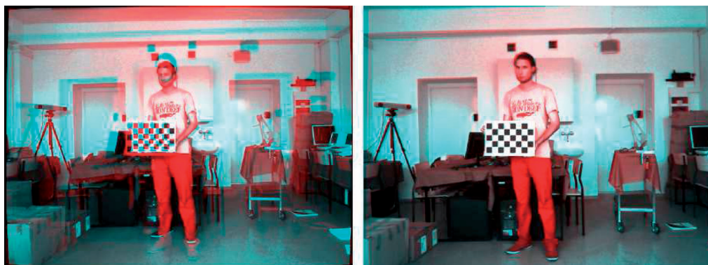
Fig. 6. Comparison of images from RGB and IR cameras before (left) and after (right) image matching and distortion removal.
