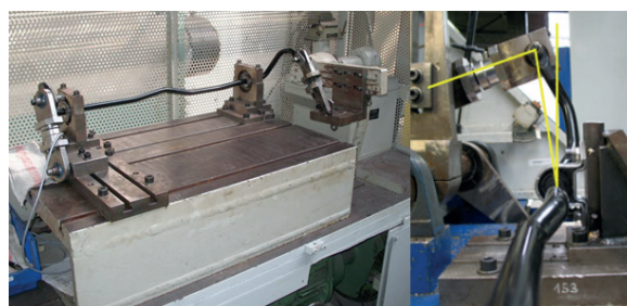
Fig. 4. Eccentric machine for dynamic tests of stabilizer bars (source TKBiS): max. dimensions of stabilizer bar: 1100 x 350 mm, diameter of stabilizer bar: 10 – 25 mm, max. forces acting on the ends of the stabilizer bar: ± 4 kN, angle of oscillation: ± 40°, frequency: 0,5 – 4 Hz
