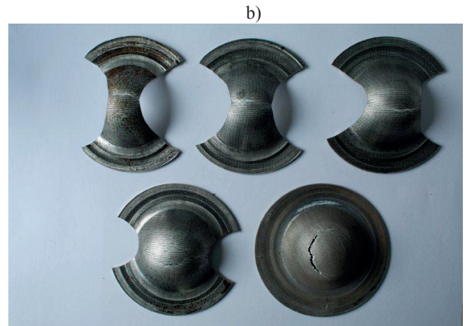
Fig. 4. Results of AZ31 alloy pressing at elevated temperatures: a) 250°C, b) 300°C – set of samples to determine FLCs
