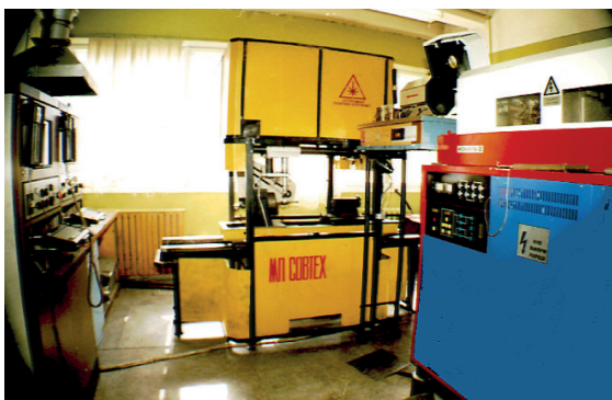
Fig. 2. Test stand of the laser hardening „Kometa-UNILAM” [22]
