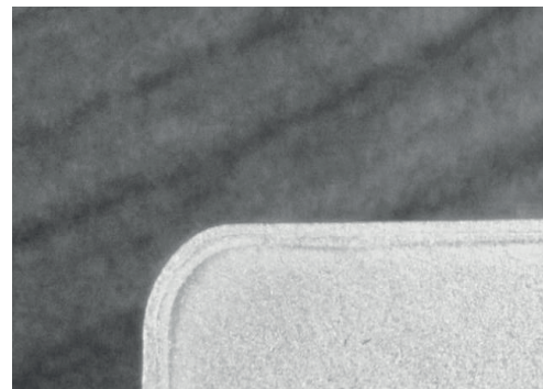
Fig. 3. Rim of coarse crystals formed during extrusion of MgAlZn alloys
