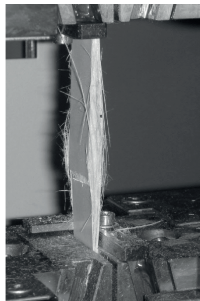
Fig. 8. Photo of the composite samples after fracture
