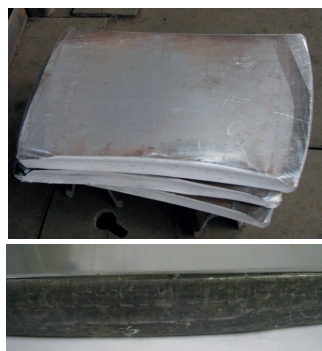
Fig. 13. Ingots of AA2519 alloy widened to ~ 600mm and prepared for rolling and cladding with EN AW-050A alloy (single-side cladding)
