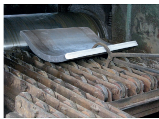
Fig. 7. Ingot widened after the cross-rolling
