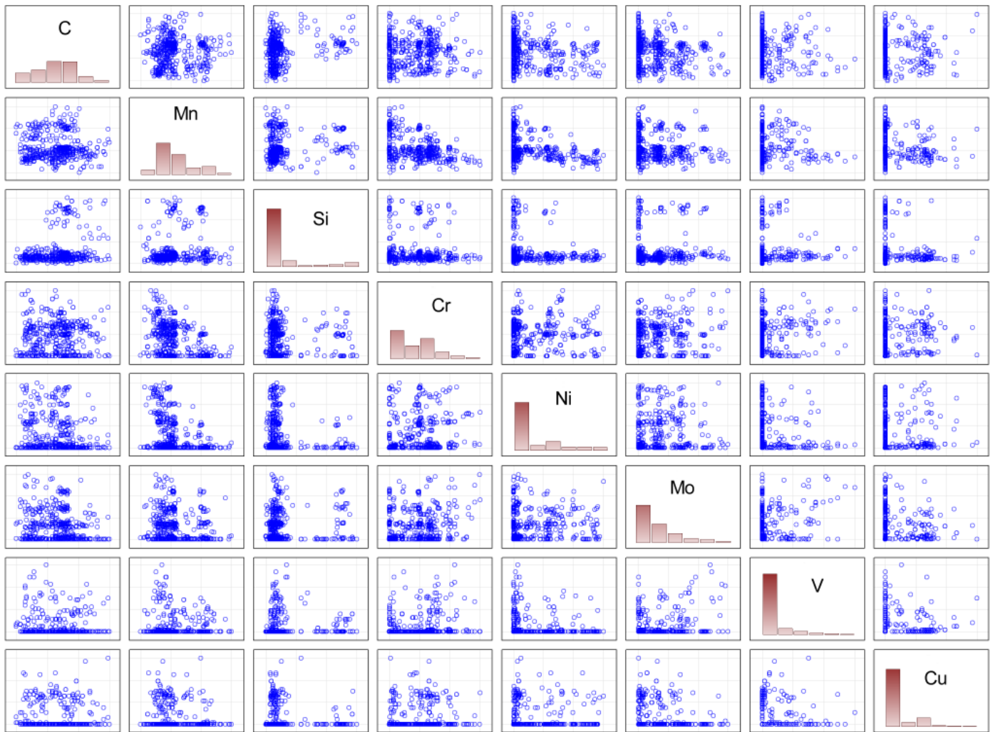
Fig. 1. Scatterplot matrix for the A_{c3} temperature model
