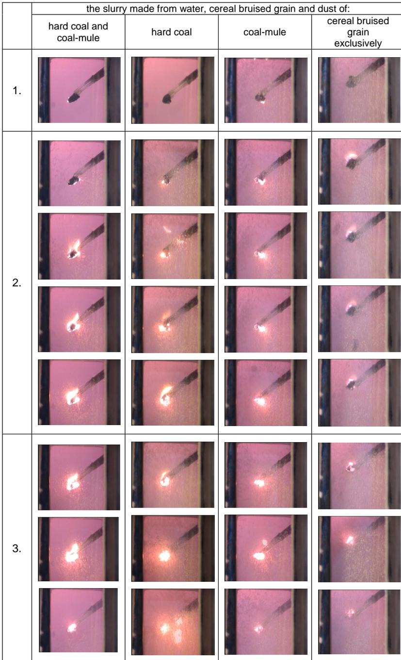
Fig. 11. Example of a course of coal-water fuel combustion process in the fluidized bed;
