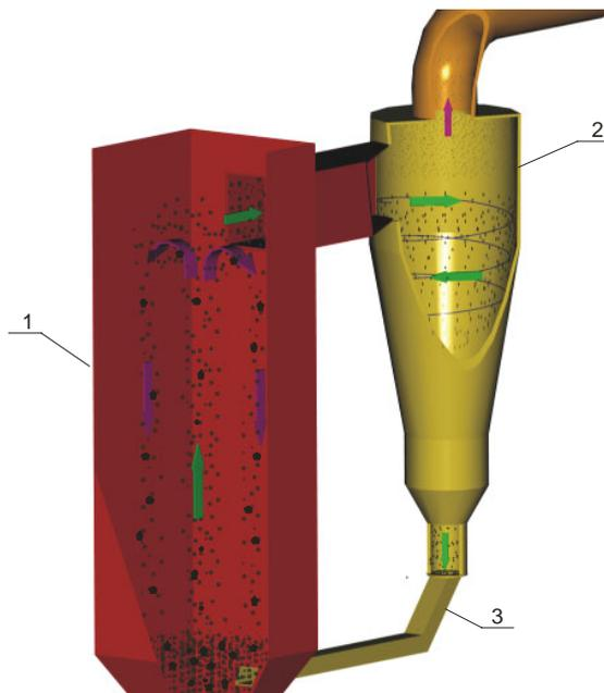
Fig. 1. Average movement of fuel particles in the boiler with a circulating fluidized bed
