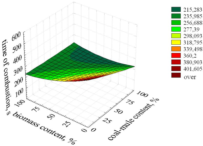
Fig. 7. The influence biomass and coal-mule content in suspension on the fuel combustion time in a fluidized bed;  $T = 850^{\circ}\text{C}$
