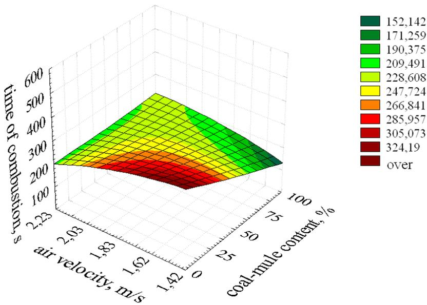
Fig. 8. The influence of air flow velocity and coal-mule content of suspension on the fuel combustion time in a fluidized bed;  $T = 850^{\circ}\text{C}$
