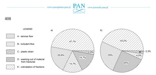
Fig. 5. Character of flow of sealing slurry with accompanying phenomena taking place in the rock mass under the influence of injected sealing slurry (a - series A, b - series Q)
