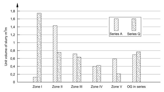
Fig. 4. Unit volume of injected sealing slurry in specific injection zones of wells of series A and Q
