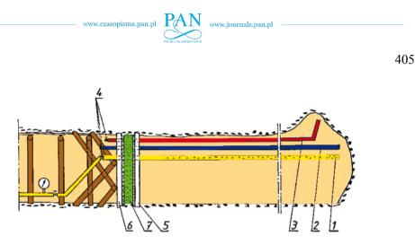
Fig. 1. Scheme of closing working's end with the pipeline injection method (1 – pumping pipeline, 2 – ventpumping pipeline, 3 – vent pipeline, 4 – gates, 5 – inner dam, 6 – outer dam, 7 – injection plug)
