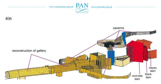
Fig. 2. Scheme of the end of the transverse working Mina
