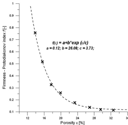
Fig. 4. The  $f$ - $\varepsilon$  relation for examined briquettes
