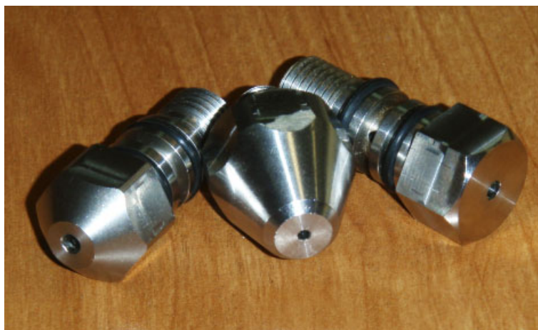
Fig. 1. STK air-and-water spraying nozzles (Pieczoza et al., 2009)
