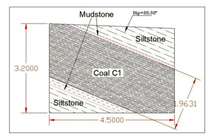
Fig. 2. Typical view of rock formations encountered in the tunnels route.
