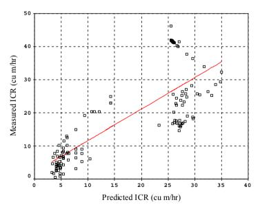
Fig. 5. Linear regression between measured and predicted ICR for all cutting cases using universal model ( $R^2 = 0.62$ )
