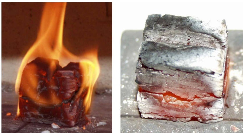
Fig. 5. Combustion of volatile matter and char particles during the tests on fracture toughness rate
