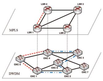
Fig. 1. MPLS over DWDM architecture
