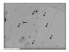
Fig. 8. BSE image of a sample SO1 (Dziewkowice limestone from Strzelce Opolskie) (Stanienda, 2013a). Magn. 2000×. Light grey – calcite. 1-6 – points of chemical analysis
