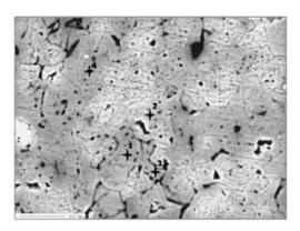
Fig. 6. BSE image of a sample SA12 (Dziewkowice limestone from Mount St. Anne) (Stanienda, 2013a). Magn. 2000×. Light grey - calcite. 1-4 – points of chemical analysis
