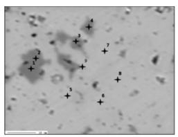
Fig. 7. BSE image of a sample S2 (Dziewkowice limestone from Szymiszów) (Stanienda, 2013b). Magn. 500×. Light grey - calcite. 1-9 – points of chemical analysis
