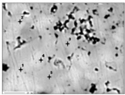
Fig. 5. BSE image of a sample SA5 (Górażdże limestone from Mount St. Anne) (Stanienda, 2013a). Magn. 2000×. Light grey – calcite; dark grey – carbonate phase rich in magnesium.
