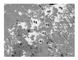
Fig. 12. BSE image of a sample TO15 (Karchowice limestone from Tarnów Opolski) (Stanienda, 2011). Magn. 1000×. Light grey – calcite; dark grey – carbonate phase rich in magnesium; white – Fe oxides. 1-6 – points of chemical analysis
