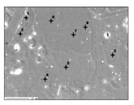
Fig. 2. BSE image of a sample G1 (Upper Gogolin limestone from Gogolin) (Stanienda, 2013a, 2014).
