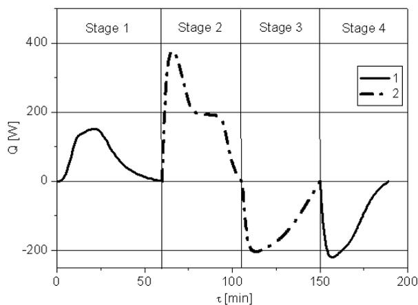
Figure 14. The heat input/output in the evaporator/condenser (1) and the low temperature carbon/BaCl<sub>2</sub> reactor (2) as a function of the cycle time.
