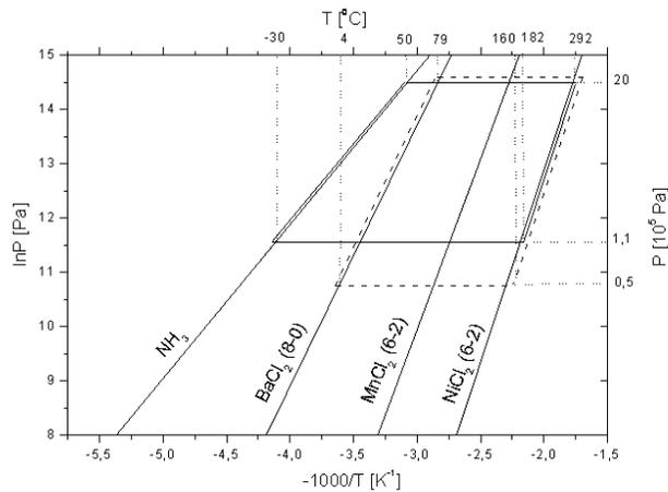
Figure 17. Clapeyron diagram for three-stage resorption heat pump (BaCl<sub>2</sub>, MnCl<sub>2</sub>, NiCl<sub>2</sub> + active carbon fibre “Busofit”) with a temperature lift near 100 °C.
