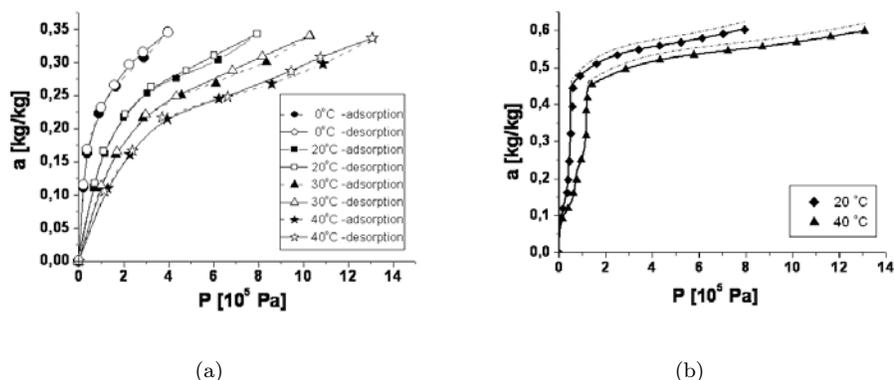
Figure 5. Dynamic ammonia sorption capacity at different temperatures vs. pressure: (a) for the active carbon fibre “Busofit” (adsorption/desorption); (b) for complex compound “Busofit”+CaCl<sub>2</sub> micro crystals (adsorption/synthesis, desorption/regeneration).
