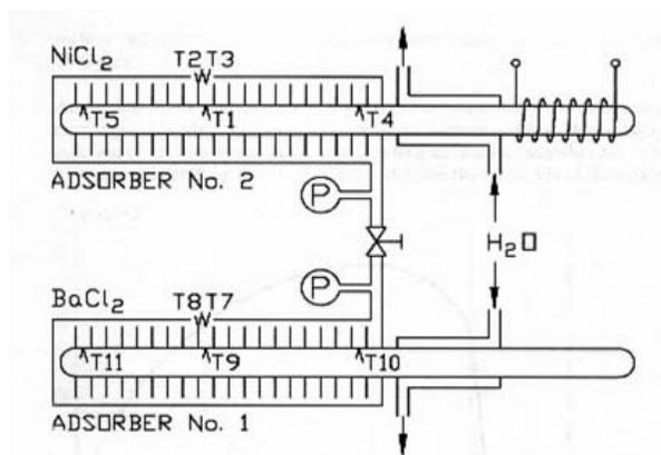
Figure 9. Sorption heat pump with two reactors ( $(\text{“Busofit”} + \text{NiCl}_2)/\text{NH}_3$ ,  $(\text{“Busofit”} + \text{BaCl}_2)/\text{NH}_3$ ) and two heat pipes for their thermal management: T1-T9 – thermocouples.
