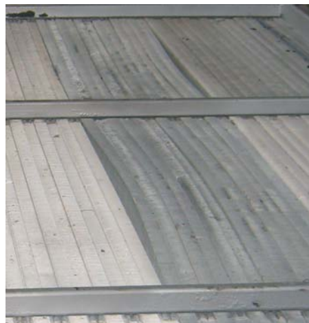
Figure 2. The buckled tube bundle.
