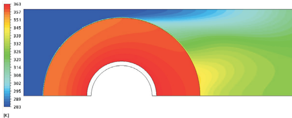
Figure 10. Temperature on fin surface and flowing air for profile (c), velocity v_{IN} = 0.5 m/s.
