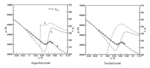
Figure 2. Pressure and temperature distributions along the nozzle.
