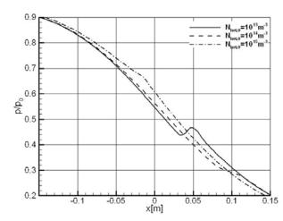
Figure 7. Effect of the soluble particles concentration on the condensation process,  $r_{p,het0} = 10^{-7}$  m.
