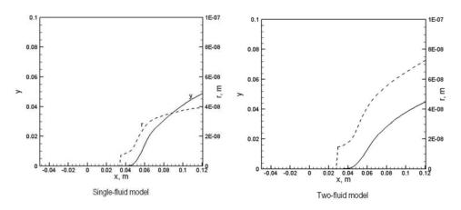
Figure 3. Wetness fraction and droplet radius distributions along the nozzle.
