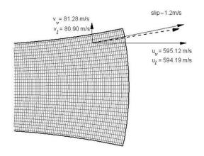
Figure 5. Slip of the velocities between vapour and liquid phase for TFM model.
