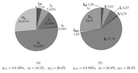
Figure 4. Split of exergy rates in the supercritical ORC power plant (a) without regeneration, (b) with regeneration.
