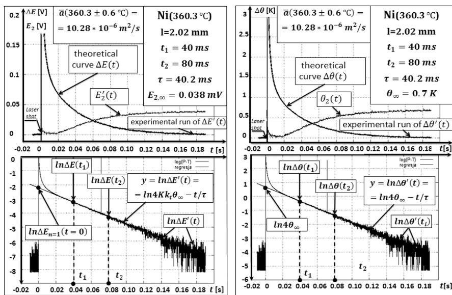
Figure 10. Thermal diffusivity results for Ni (99.9% wt) at the temperature of  $T = 360.3 \text{ }^\circ\text{C}$ , and runs of the temperature changes  $\Theta_2(t)$  and  $\Delta\Theta(t)$ .
