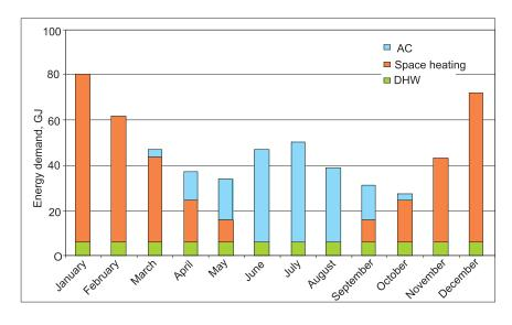
Figure 1. The energy demand of a small office building, located in Warsaw [8]: AC – air conditioning, DHW – domestic hot water.
