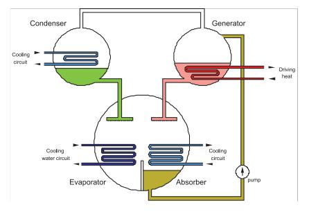
Figure 5. Absorption refrigeration device.
