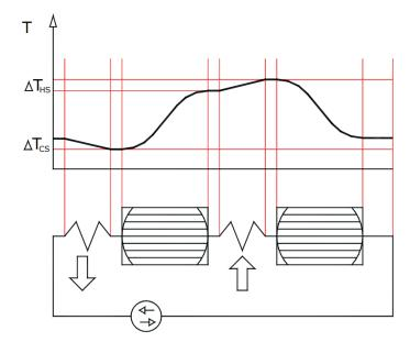
Figure 11. Working fluid temperature in thermal wave adsorption system.
