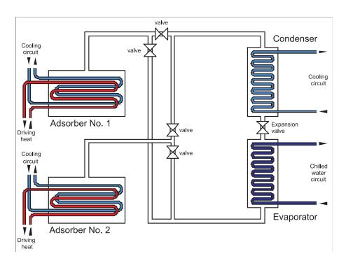
Figure 6. Adsorption refrigeration device.
