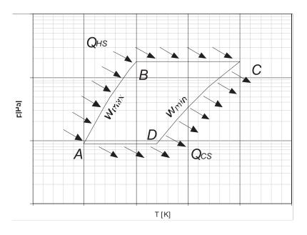
Figure 8. Adsorbers thermodynamic states.
