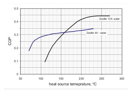
Figure 9. Coefficient of performance as function of driven heat source.
