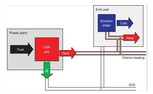
Figure 3. Centralized trigeneration system with decentralized cold generation.
