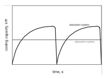
Figure 7. Cooling capacity as a function of the time.
