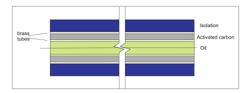
Figure 12. Adsorber cross-section.
