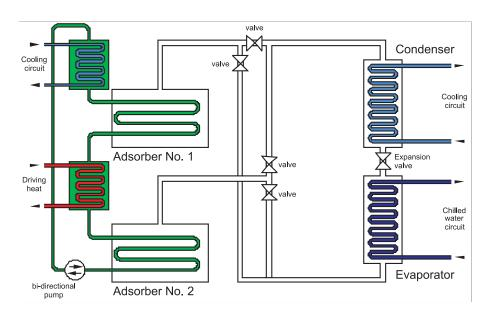
Figure 10. Thermal wave adsorption system.  $\,$
