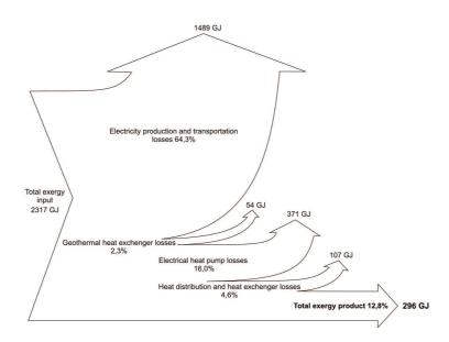
Figure 5. Exergy flow diagram of the system with electrical heat pump.
