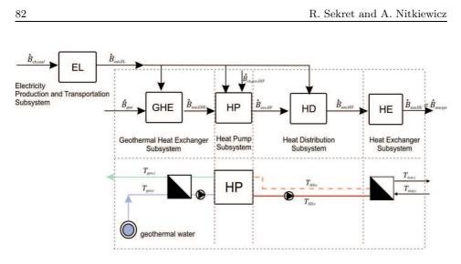
Figure 4. Schematic diagram of exergy flow in the heating system.
