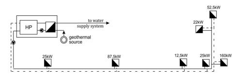
Figure 1. The concept of low temperature geothermal district heating system: HP – heat pump, white/black square – heat exchanger.
