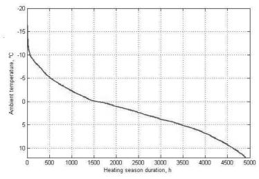
Figure 2. Ambient temperature time characteristic for typical heating season.
