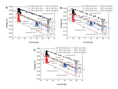
Figure 8: The effect of the CBFC on I-V characteristic with the various operating temperatures at 750 and 730  $^{\circ}$ C for keeping the fuel utilization factor at: A) 50%, B) 60% and C) 70%.
