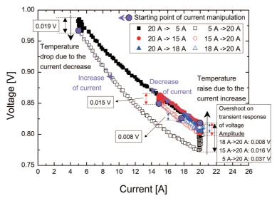
Figure 4: Transient current-voltage (I-V) characteristic with a variety of current changes at the open fuel utilization factor condition.
