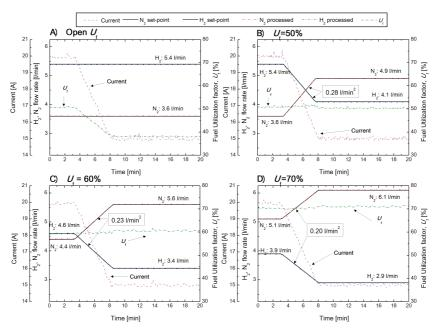
Figure 2: Manipulation of fuel flow rate in order to keep the fuel utilization factor: A) fixed (the so-called open fuel utilization factor), B) 50%, C) at 60% and D) at 70% during the current changed from 20 to 15 A at a rate of 1 A/min.
