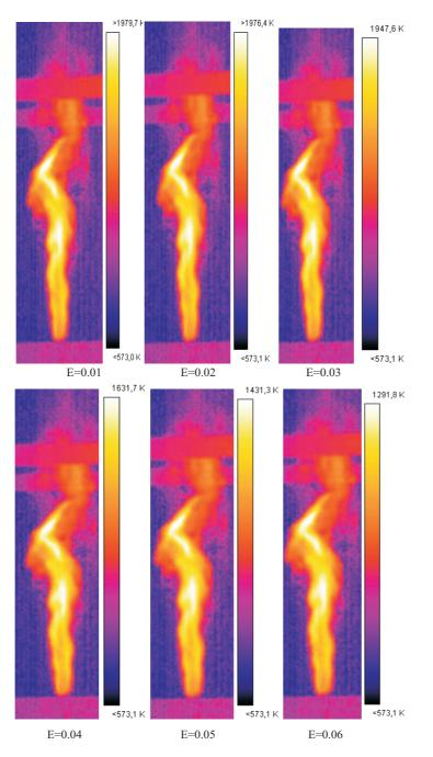
Figure 7: Methane diffusion flame contour for different flame emissivity, E, (thermography results).
