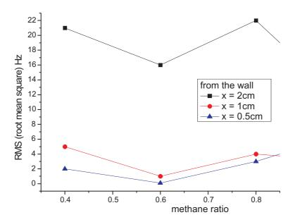
Figure 6: Root mean square RMS value for combined effect of nitrogen dilution rate and the impinging wall.
