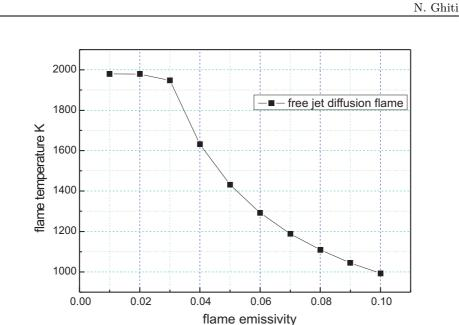
Figure 8: Temperature of methane diffusion turbulent flame as a function of flame emissivity (at Reynolds number of 6000).
