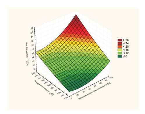
Figure 3: Dependency of the impact of humidity W = 10-60% and flue gas temperatures  $t_{fg} = 120 \,^{\circ}\text{C}$  and  $200 \,^{\circ}\text{C}$  on the extent of heat flue gas loss in the heat generator  $\xi_k$ .
