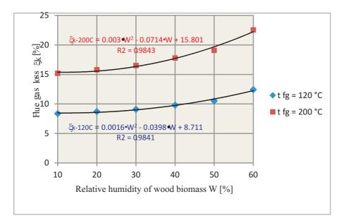
Figure 2: The dependence of flue gas loss on the humidity of wood biomass for flue gas temperature of 120  $^\circ \rm C$  and 200  $^\circ \rm C.$
